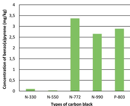
**Fig. 3.** Concentration of benzo(a)pyrene in carbon blacks
