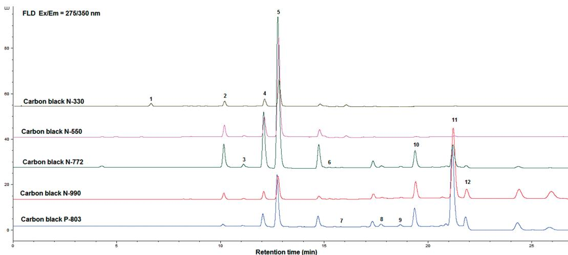
**Fig. 1.** HPLC-FLD chromatograms of PAHs extracted with hexane in carbon black N-330, N-550, N-772, N-990 and P-803 Identified PAHs: (1) naphthalene, (2) phenanthrene, (3) anthracene, (4) fluoranthene, (5) pyrene, (6) benzo(a)anthracene, (7) chrysene, (8) benzo(b)fluoranthene, (9) benzo(k)fluoranthene, (10) benzo(a)pyrene, (11) benzo(g,h,i)perylene, (12) indeno(1,2,3-cd)pyrene
