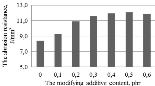
Fig. 2. The abrasion resistance of the elastomeric compositions, containing PTFE pyrolysis product
