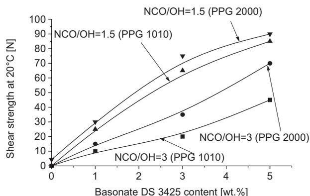
Figure 8. Effect of concentration of Basonate FDS 3425 on shear strength of polyurethane PSA
