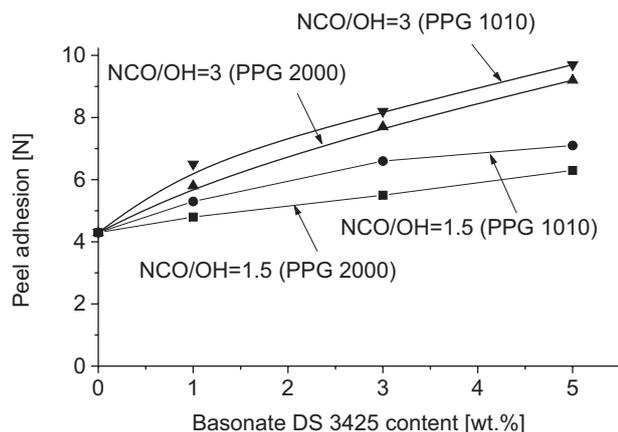
Figure 7. Effect of multifunctional isocyanate Basonate FDS 3425 amount on the peel adhesion of polyurethane PSA
