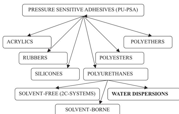
Figure 1. Polymer types for manufacturing of pressure sensitive adhesives
