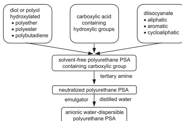
Figure 4. Synthesis schemas of water-borne polyurethane self-adhesives
