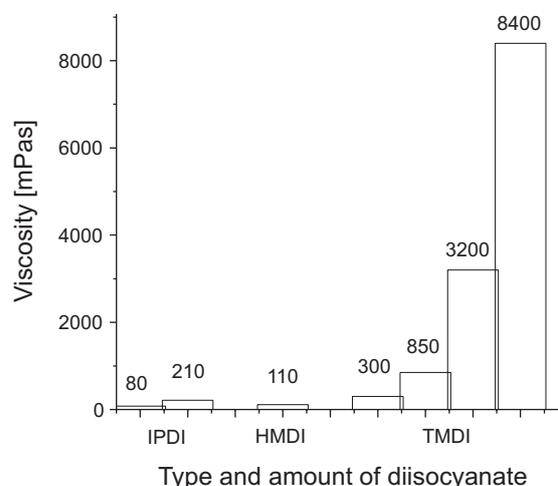
Figure 6. Viscosity of synthesized water-borne PU-PSA
