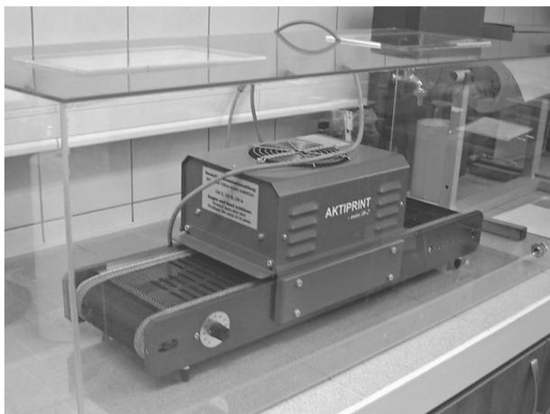
Figure 3. UV-lamp AKTIPRINT-mini 18-2 from Technigraf with mobile band
