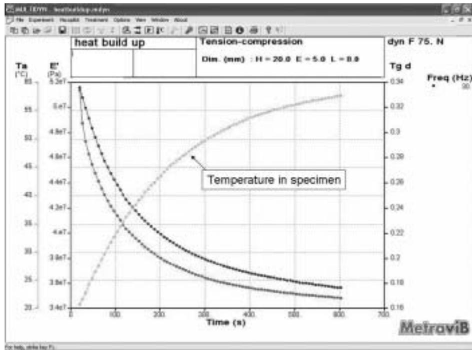
Figure 12. *Elastomer – Heat build up phenomenon.*
