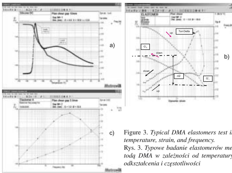
Figure 3. Typical DMA elastomers test in temperature, strain, and frequency.
