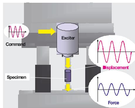
Figure 4. Classical DMA principle
