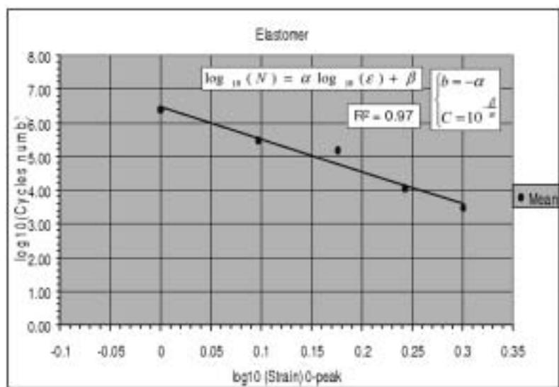
Figure 15. Post processing of the equivalent of Basquin's ratio for the elastomer tested.
