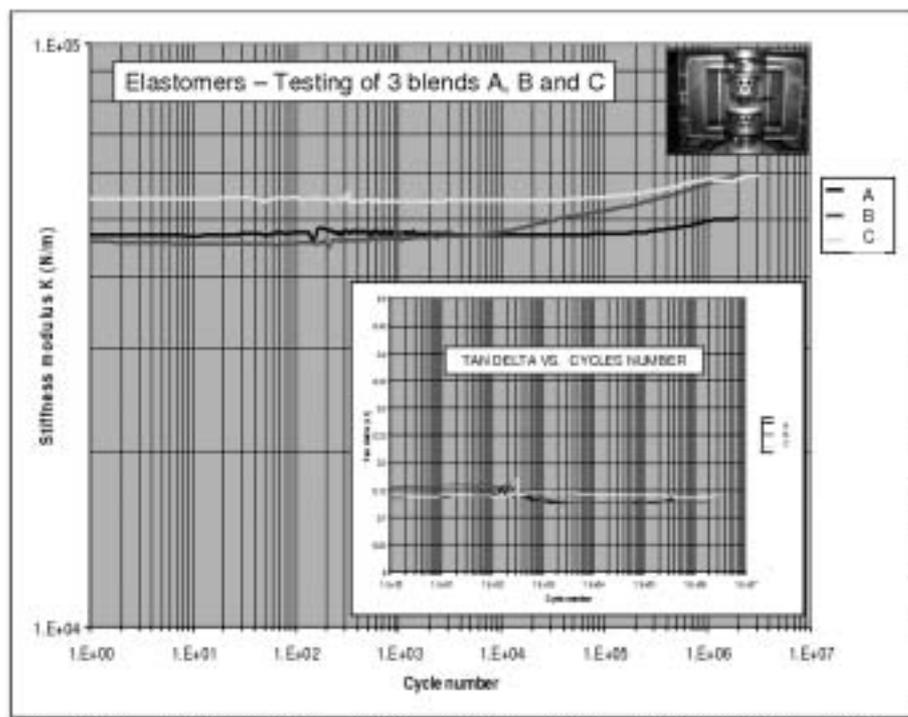
Figure 13. *Testing in fatigue of 3 elastmer blends used for the same type of final application.*
