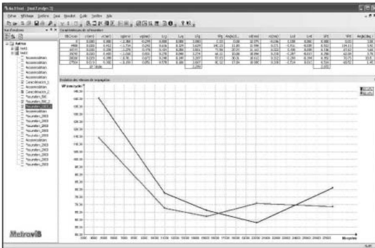
Figure 17. Elastomer – Crack growth measurement – Crack growth speed in nm/cycles vs. cycles number.
