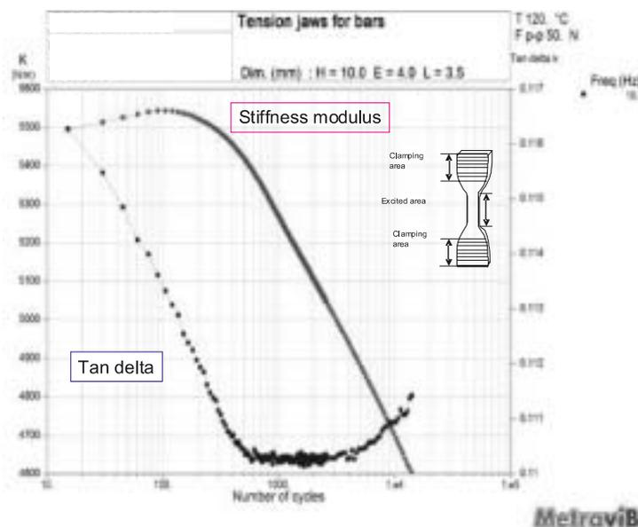
Figure 14. Elastomer – Fatigue test with MULTITEST up to the breaking of the specimen at a given strain.
