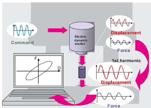
Figure 5. Typical control loops in a classical DMA test
