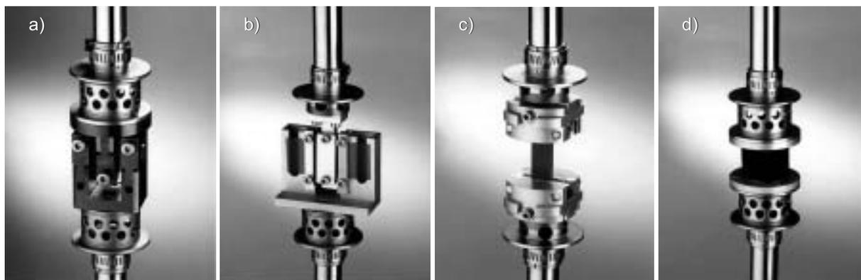
Figure 2. Specimen holders currently used for elastomers testing: a) shear for sandwiches, b) shear for films, c) tension jaws, d) compression plates
