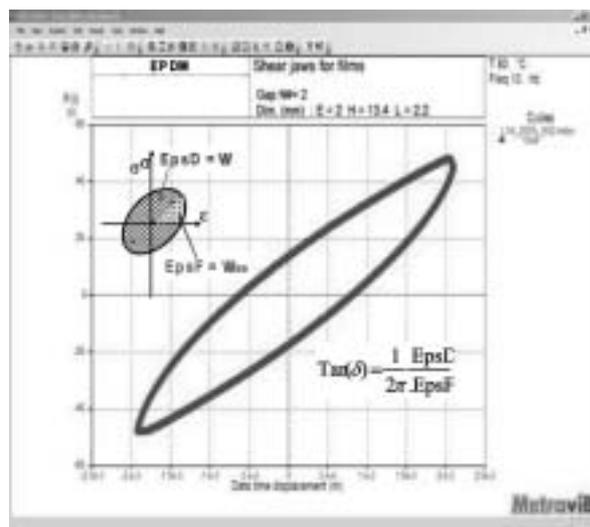
Figure 8. Loss factor  $\tan \delta$  determined from one hysteresis loop.
