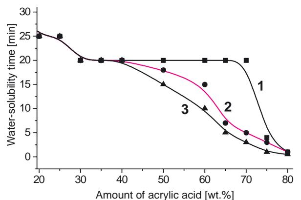
Fig. 2. The influence of acrylic acid amount in the polymer on its time of water solubility time: 1 – pH = 4; 2 – pH = 7; 3 – pH = 11
