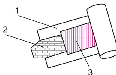
Fig. 9. Design of new biomedical electrode; 1 – carrier, 2 – electrically conductive film, 3 – acrylic PSA
