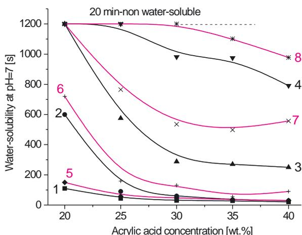
Fig. 3. Effect of crosslinkers AlACA and ZrACA on water-solubility of acrylic PSA at pH=7: 1 – 0.5% AlACA, 2 – 1% AlACA, 3 – 1.5% AlACA, 4 – 2% AlACA, 5 – 0.5% ZrACA, 6 – 1% ZrACA, 7 – 1.5% ZrACA, 8 – 2% ZrACA
